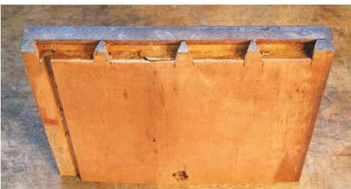
◀ Pic.1 An old lapped dovetail pinboard (aka drawer front) with planted-on lipping. Notice how the groove for the drawer bottom comes out in a tail so that it is not seen. Notice also the half pins at the outside edges
